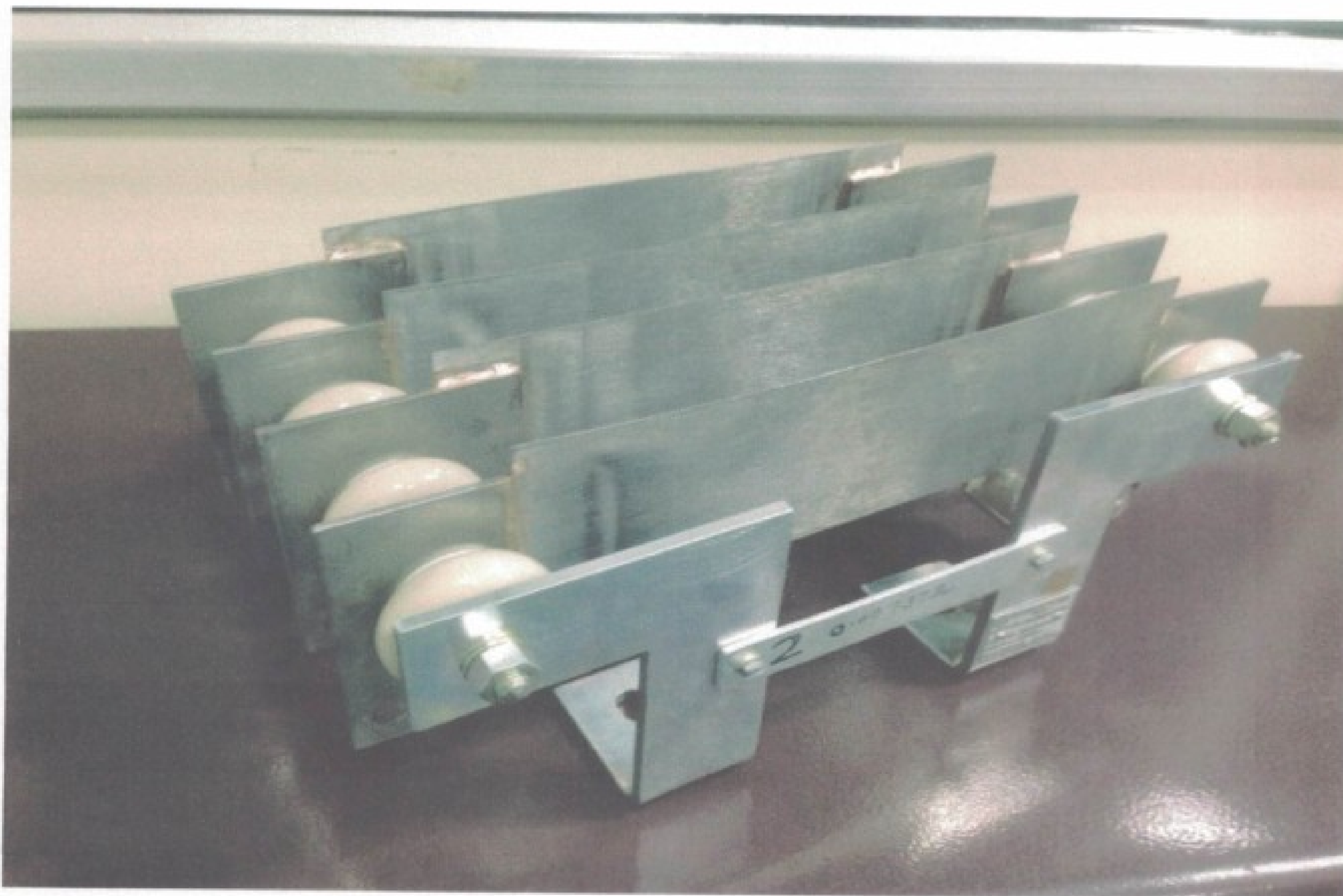
FIELD SHUNTING RESISTOR FOR MGDE
